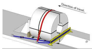
Frame straps must be anchored a minimum of 500 mm from rear face of coil (see 4.1 and 4.2).
